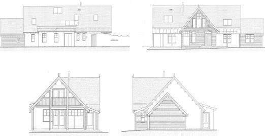
Fig. 8 - New elevations (changes: smooth render and slate)
