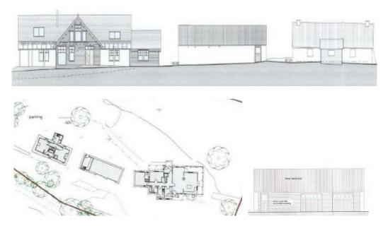
Fig. 6 & 7 – Main (south) elevation and site layout showing repositioned dwelling and retained steading with alterations
